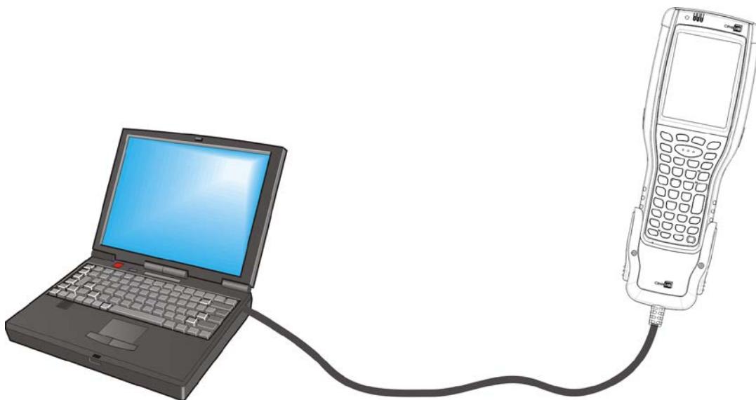
Figure 11: Direct Data Communication Using Snap-on Cable
